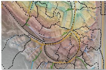
The tool will use the latest land use and soil maps in conjunction with the catchment delineations to develop hydrologic parameters. Catchments will be developed and analyzed for existing and future general plan land use.
