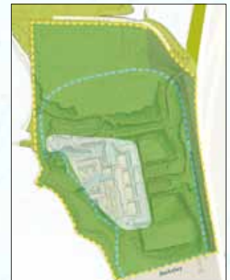
This diagram shows Concept #6 with not more than 27 acres of built area (including parking, circulation, roads, interior open spaces, etc.) within the allowable development boundary area (blue dotted line).
