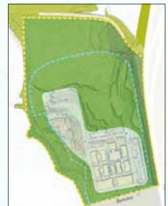
This diagram shows Concept #3 with not more than 27 acres of built area (including parking, circulation, roads, interior open spaces, etc.) within the allowable development boundary area (blue dotted line).
