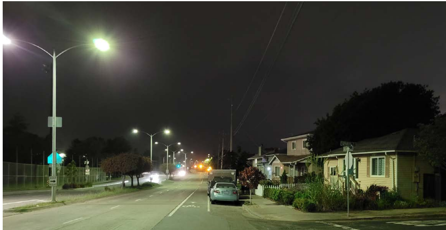
LIGHT TRESPASS FROM EXCESSIVE STREET LIGHTING
