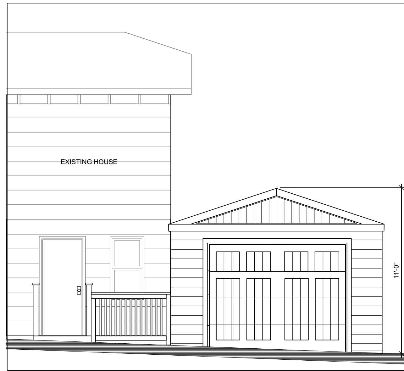
A PROPOSED GARAGE WEST ELEVATION 5 Scale: 1/4" = 1'-0"
