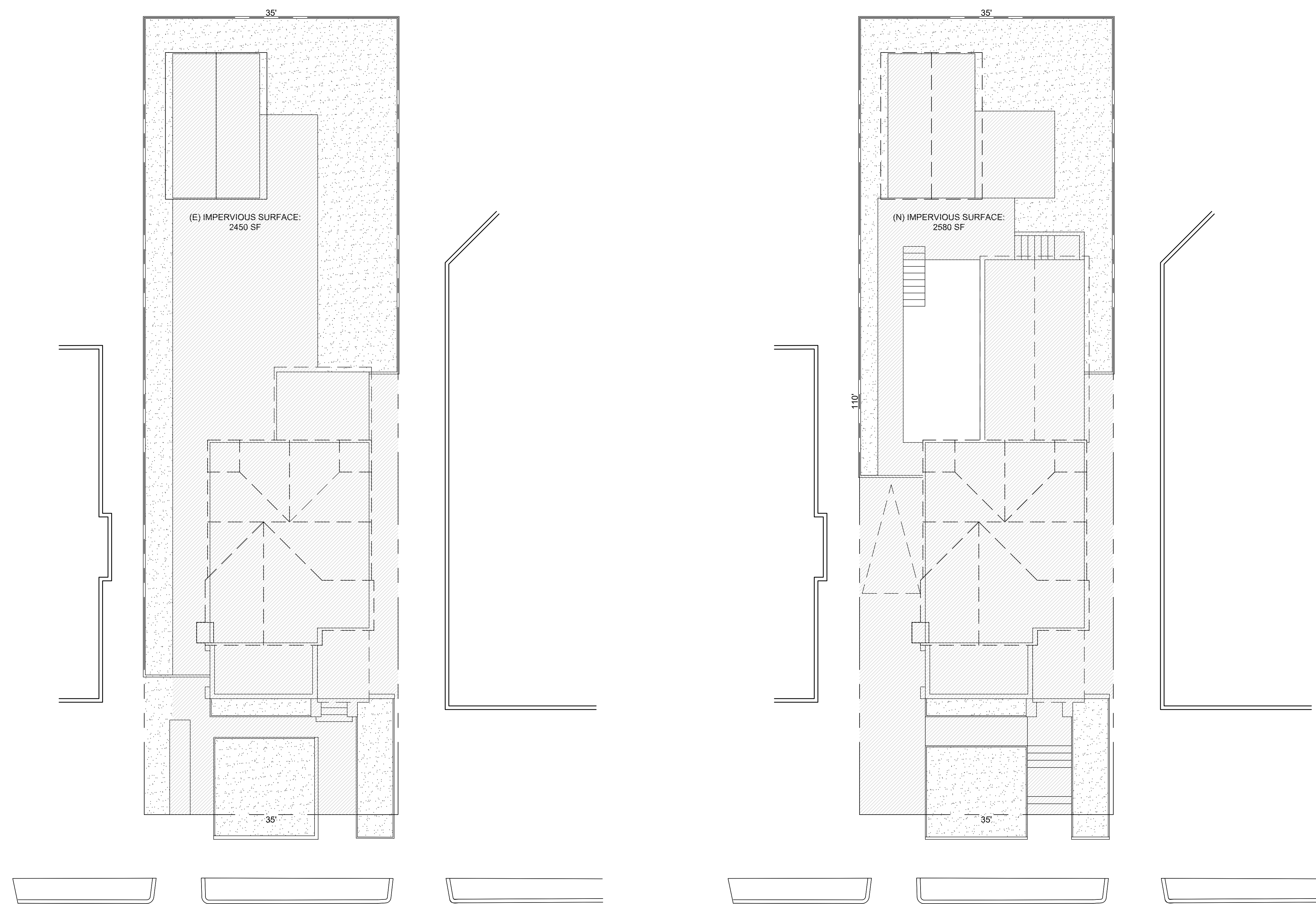
2 EXISTING IMPERVIOUS SURFACE SCALE 1/8" = 1'-0"
