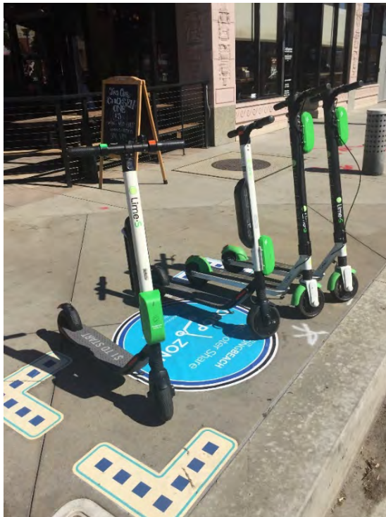
Figure 2.10. Scooter parking pads in Long Beach, CA. These pads are removable and can easily be relocated based on demand.
