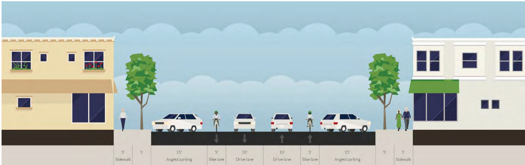
Figure 2.8. Potential Solano Avenue cross section with Class II bicycle lanes and angled parking on westbound and eastbound sides.
