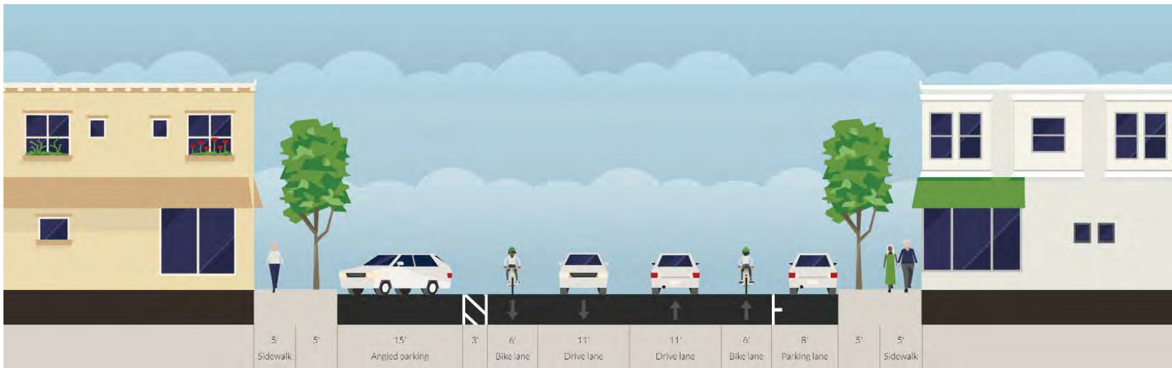
Figure 2.9. Potential Solano Avenue cross section with Class II bicycle lanes and angled parking on westbound side and parallel parking on eastbound side.
