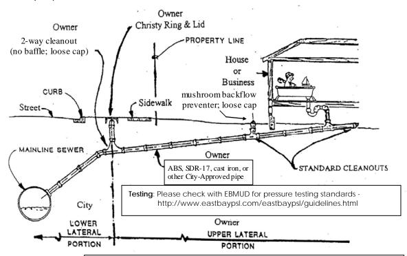
**NOTE**: Cleanouts and portions of sewer lines underneath a driveway or driveway approach must be cast iron.
