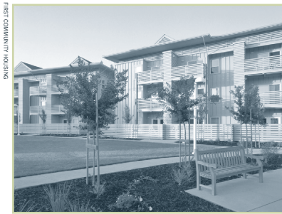
The courtyard at Betty Ann Gardens affordable apartments in San Jose has many elements for natural surveillance: balconies that look toward a central area, benches to encourage leisure time, and proper site lighting.
