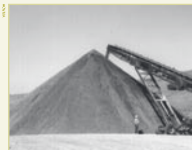
Concrete from construction and demolition practices is crushed and turned into recycled aggregate.
