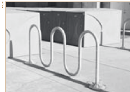
Wave racks with wide spacing between slots will accommodate more bikes than narrow racks. Individual lockers offer the most security.
