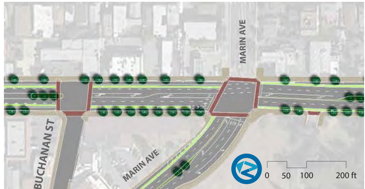
Figure 3-19 Option 3 - Example Transition from Bike Lanes to Shared Lane Markings on San Pablo
