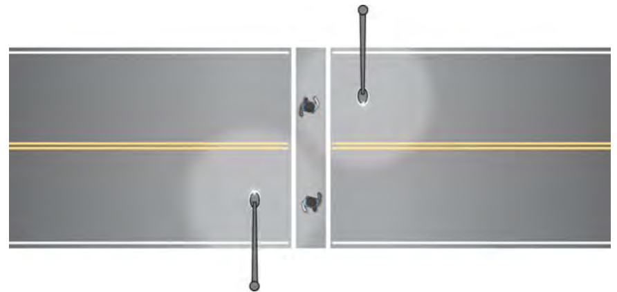
Figure 3-3 Pedestrian Lighting at Crosswalks Graphic
