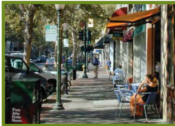
Street lights should illuminate the sidewalk at the pedestrian scale and also meet roadway illumination requirements. (Palo Alto, CA)
