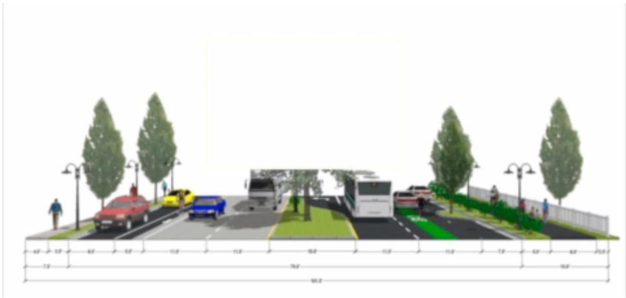
Photo 15: Proposed cross-section of Buchanan Street
