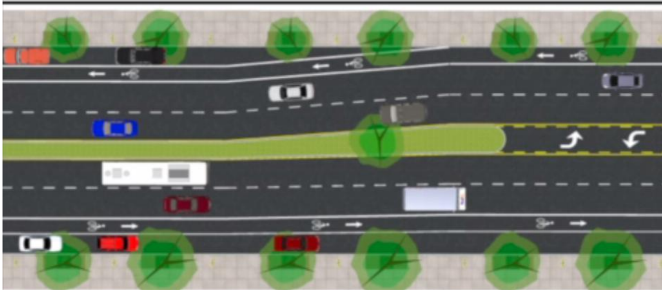
Photo 6: Cross section of Option 2 on San Pablo Avenue that shows the transition between a median and no median with left-turn lane
