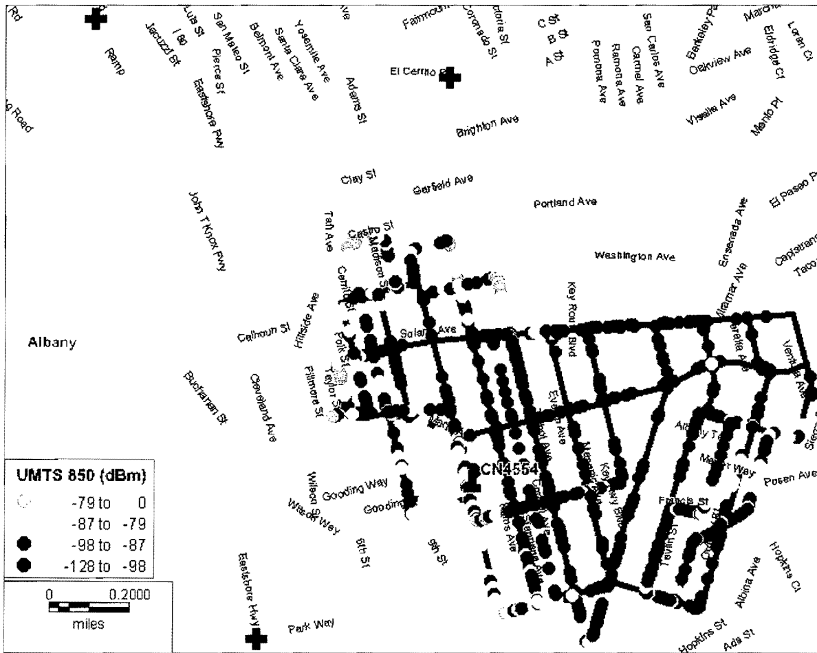
Figure 4 – Witnessed Drive Test Results (870 MHz Band)
