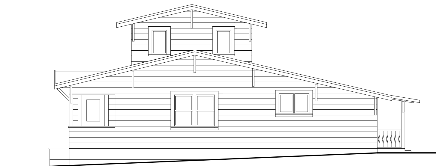
NORTH/SIDE ELEVATION Scale: 1/8" = 1'-0"
